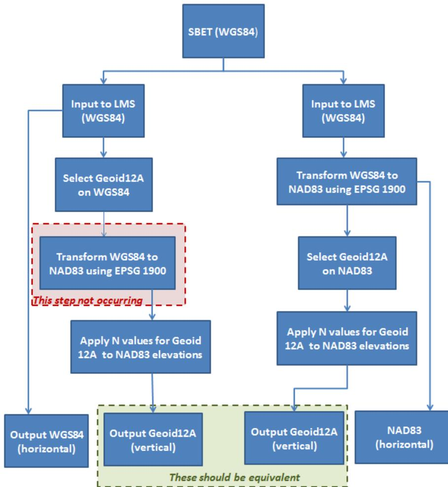
**Figure 3** - Flow chart of troubleshooting processes in LMS. Left hand side of the flow chart indicates the typically processing flow and the step in which the error is introduced. Right hand side of the flow chart shows the process followed for producing comparable elevation results.
