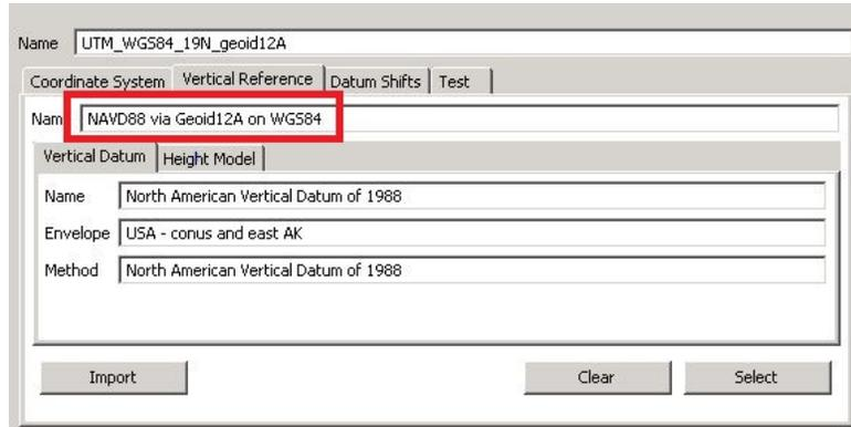
**Figure 2.** Option selected in LMS for transforming WGS84 ellipsoidal heights to Geoid12A ortho-metric heights
