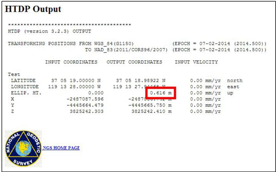
Figure 6. Results of HTDP output with corrective shift highlighted
