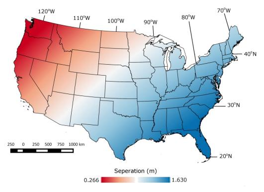
Figure 4. Vertical separation between WGS84 (G1150) and NAD83 within the contiguous United States
