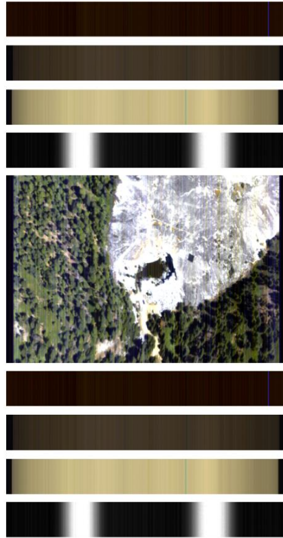
Figure 8: Example of a NIS OBC collect. In this figure, time is increasing from the top down. Each of the OBC collects have been temporally shortened for illustration. The OBC data is used for verification of the NIS behavior during the science collect.
