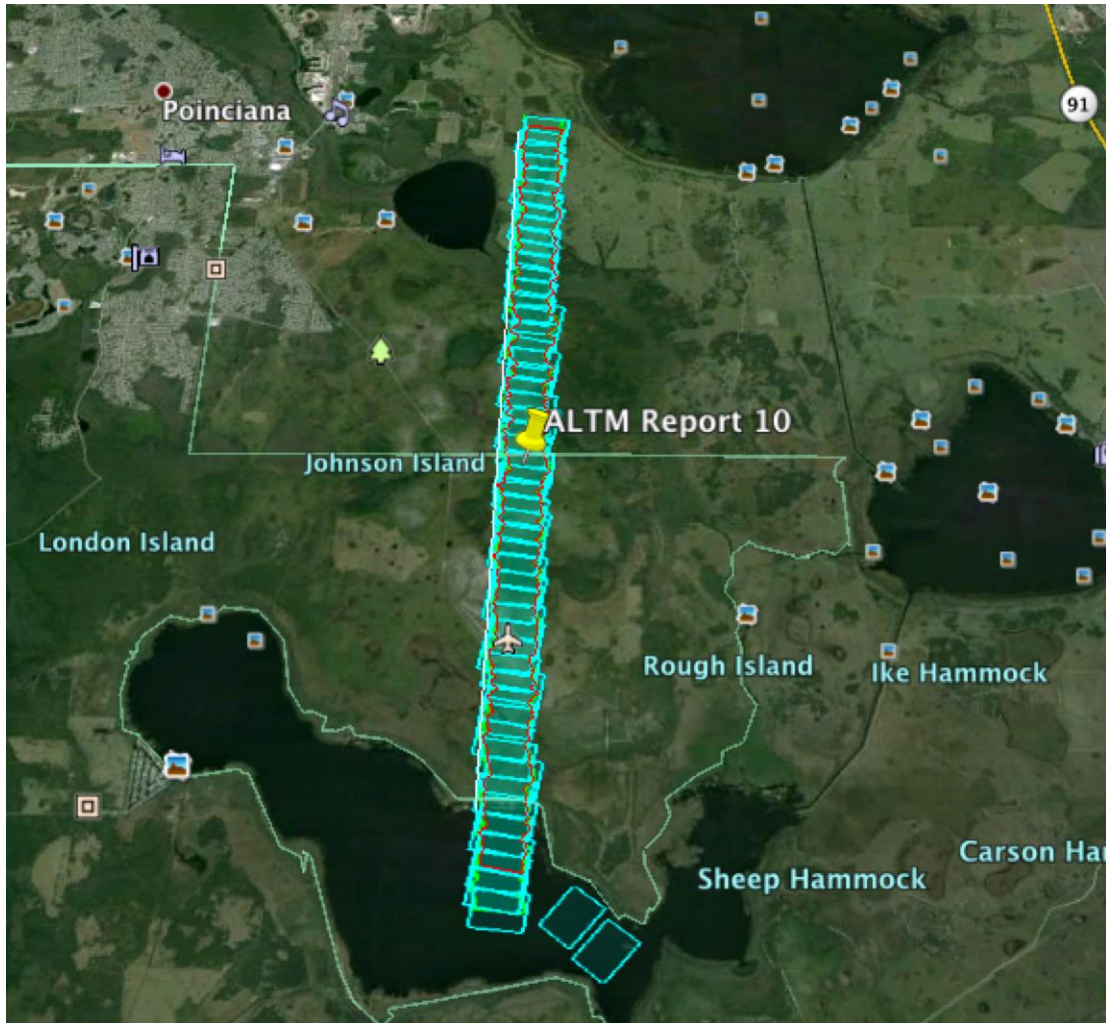
Figure 24: Photo (light blue), LiDAR (green), and spectrometer (red) coverage polygons for a single flight line over DSNY from 2014
