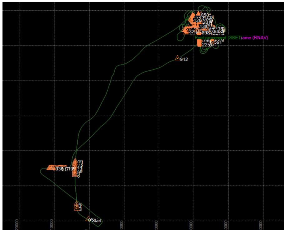
Figure 7: Processed trajectory which shows successful combination of GPS and IMU data
