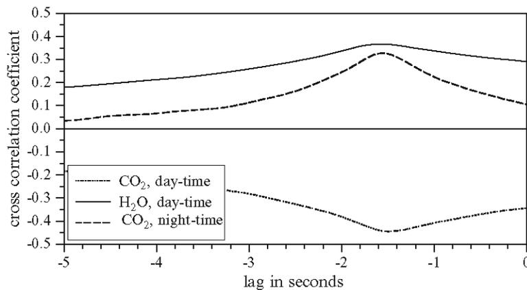
Figure 4. From Rebmann et al. (2012): Cross-correlation between the vertical wind component and CO<sub>2</sub> and H<sub>2</sub>O for different lag times.
