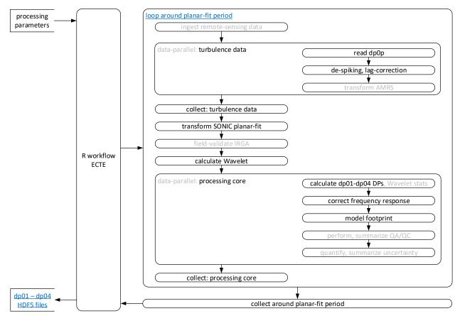
Figure 7. The EC turbulent exchange workflow within the eddy4R-Docker EC processing framework (Sect. 4).
