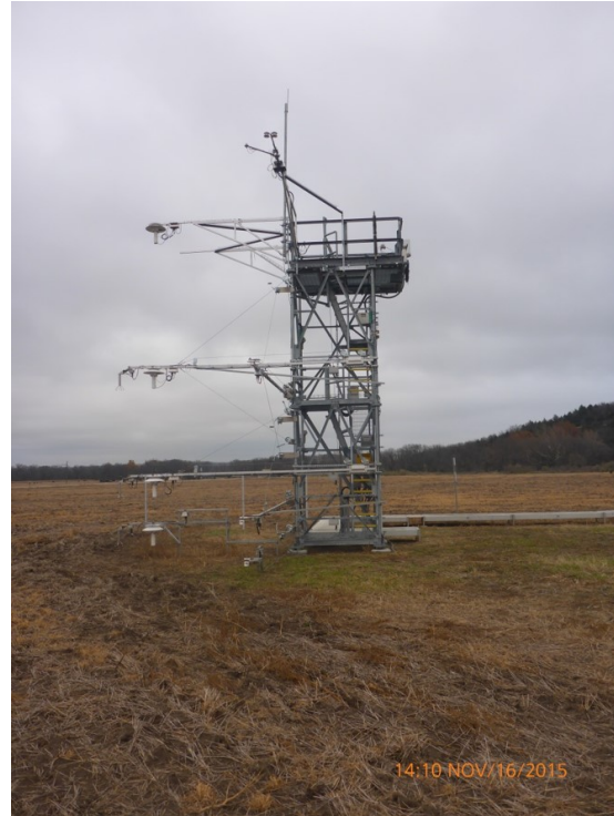
Figure 14. The NEON tower design. Left panel: conceptual design and location of individual instrument assemblies for a 4-level tower: 2D sonic anemometer (T01, T03, T05), air temperature sensor (T02, T04, T06, T07), eddy covariance boom (T08; including 3-D sonic anemometer, infrared gas analyzer, attitude and motion reference sensor), environmental enclosure (T09), secondary precipitation gauge (T10), spectral photometer (T11), radiation boom (T12), pyranometer (T13), sunshine pyranometer (T14), net radiometer (T15), up-facing and down-facing PAR sensors (T16), mid-level radiation boom (T17, T18, T19; including an up-facing PAR sensor and an infrared temperature sensor). Right panel: example of a 4-level tower at NEON CPER site.
