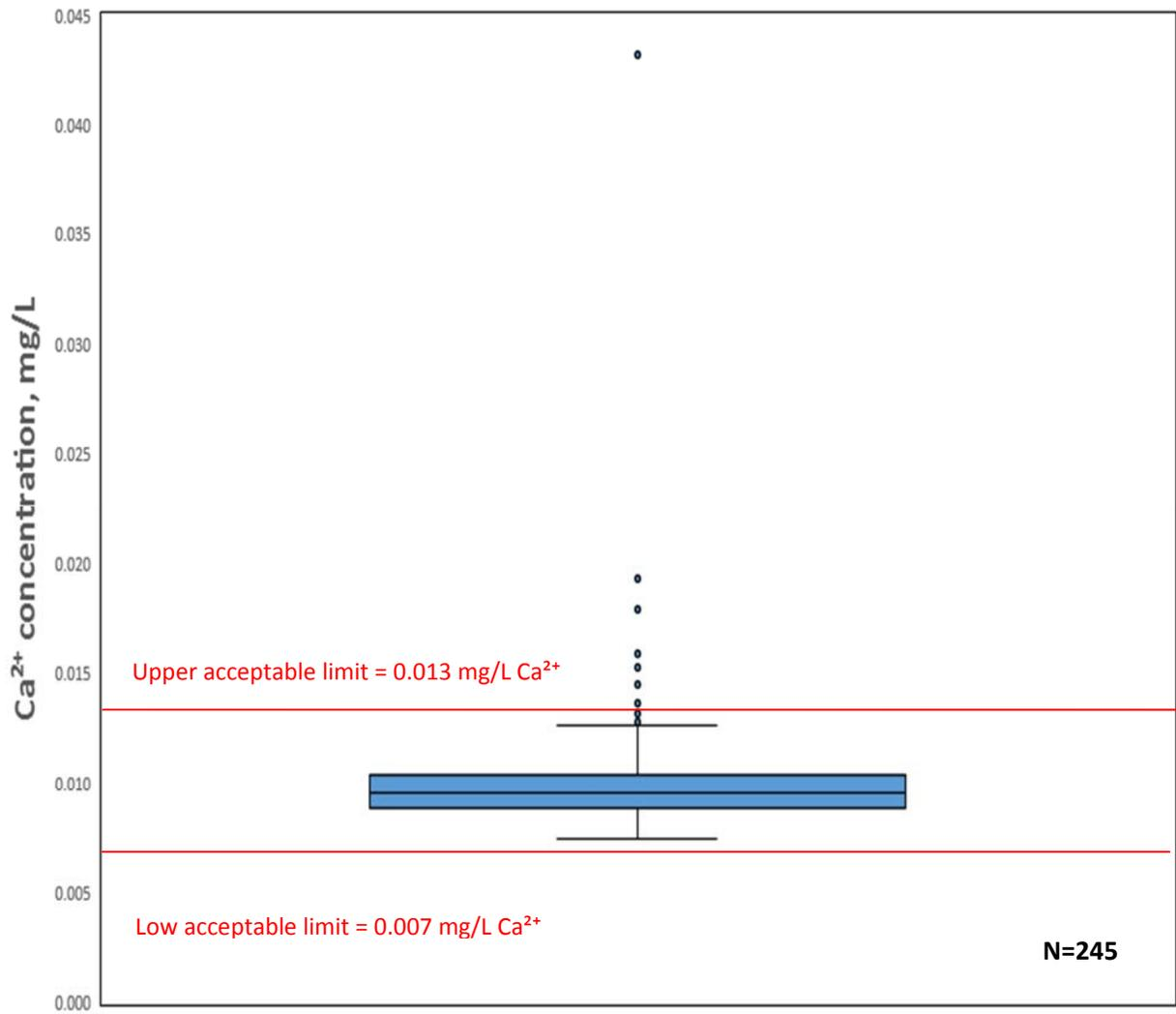
Figure 5. Box and whisker plot showing Ca<sup>2+</sup> concentrations for washed and reused buckets, tested with MDL solution in 2016
