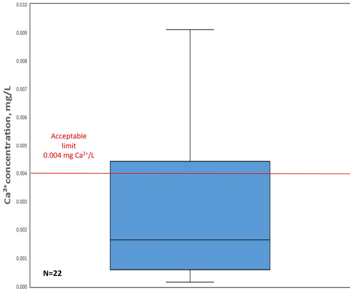
Figure 7. Box and whisker plot showing Ca<sup>2+</sup> concentrations for new lids, tested with DI water in 2016
