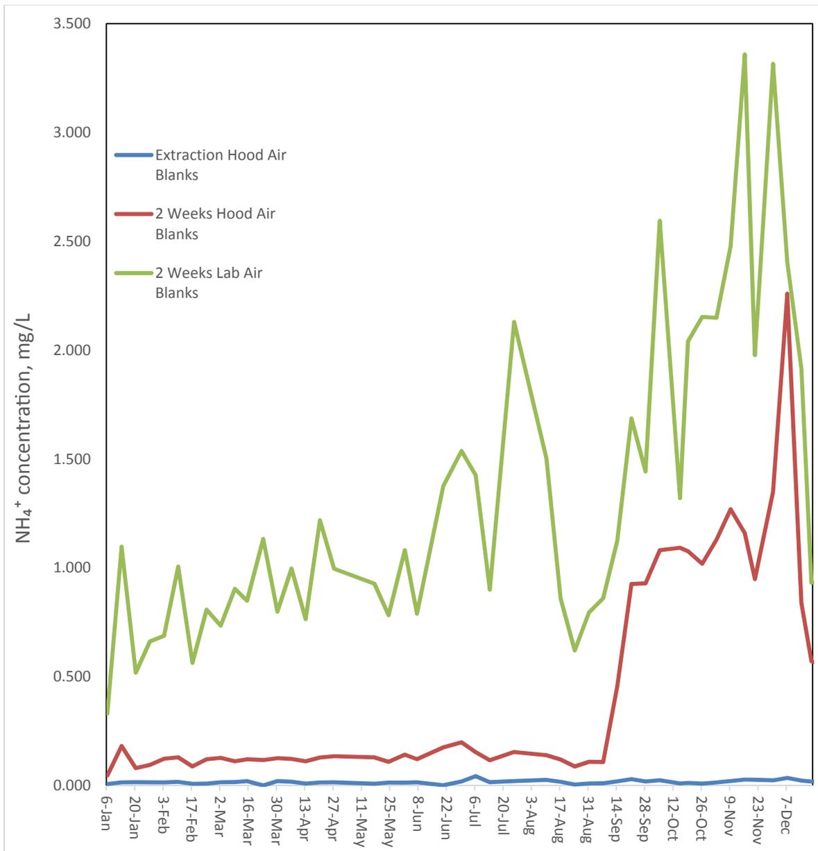
**Figure 11. Comparison of lab air blanks ( $\text{NH}_4^+$  concentrations, measured in 2016 in hood air blanks during extraction, two week hood air blanks and two week lab air blanks)**
