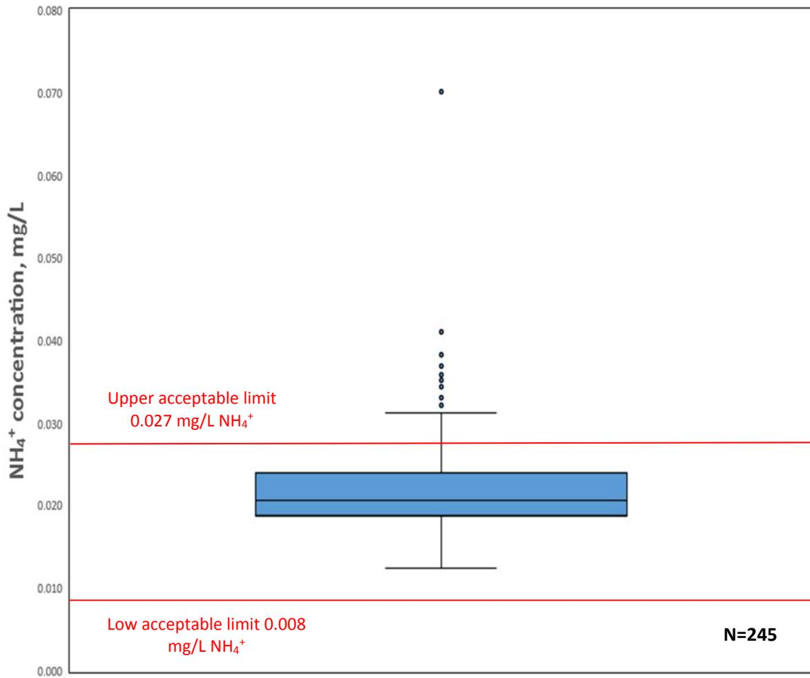
Figure 10. Box and whisker plot showing  $\text{NH}_4^+$  concentrations for washed and reused bucket lids, tested with MDL solution in 2016
