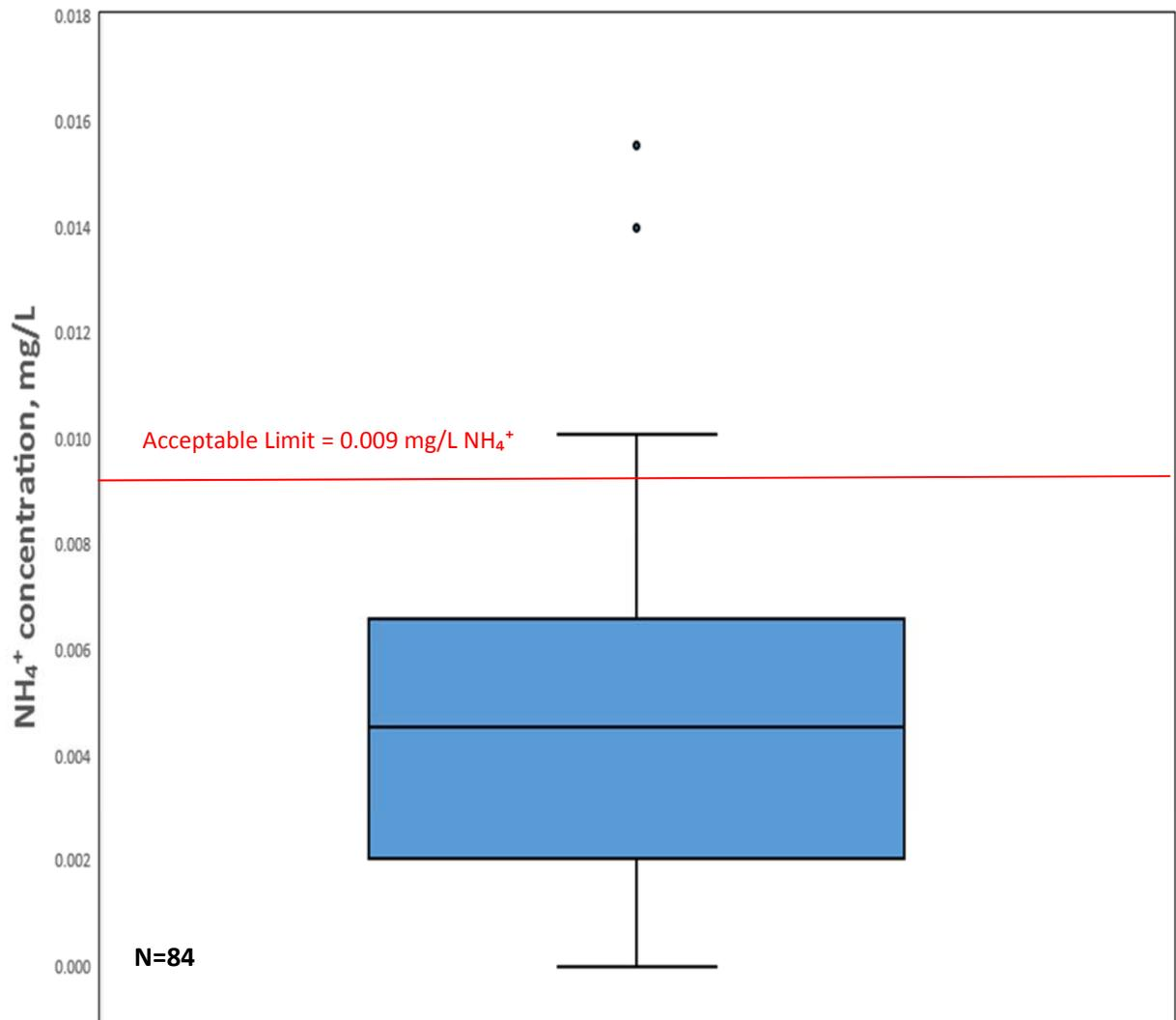
Figure 4. Box and whisker plot showing  $\text{NH}_4^+$  concentrations for new buckets, tested with DI water in 2016
