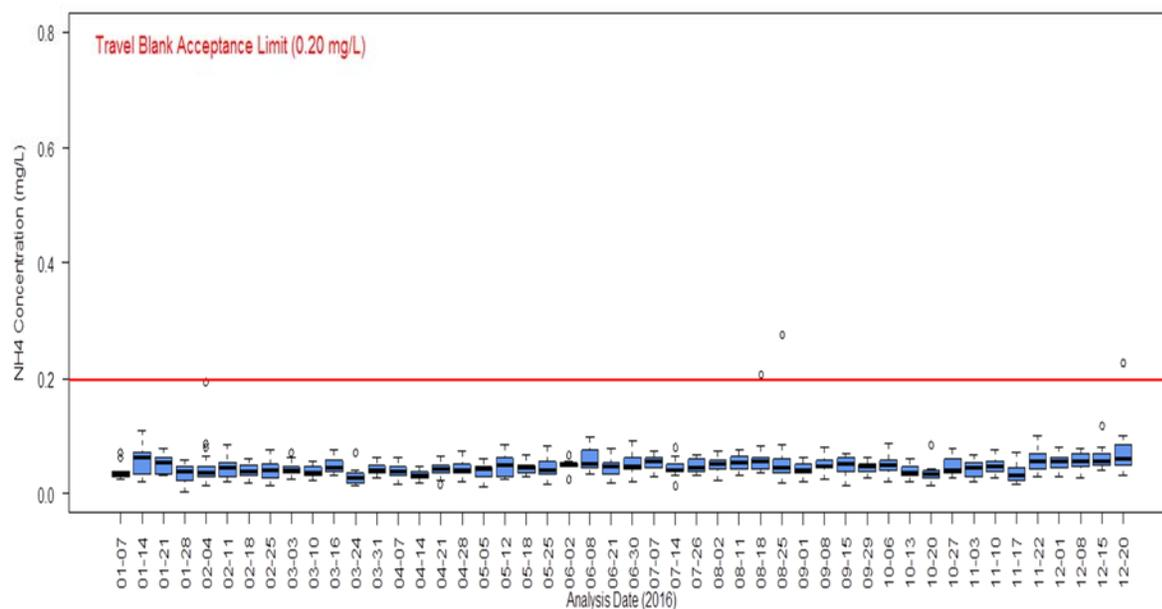
**Figure 15. Box and whisker plot showing ammonium ( $\text{NH}_4^+$ ) concentrations in extracts of AMoN travel blanks in 2016, grouped by analysis date**
