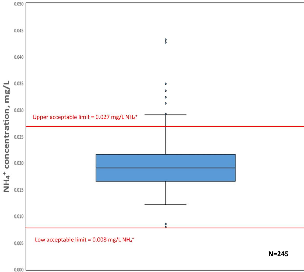
Figure 6. Box and whisker plot showing  $\text{NH}_4^+$  concentrations for washed and reused buckets, tested with MDL solution in 2016
