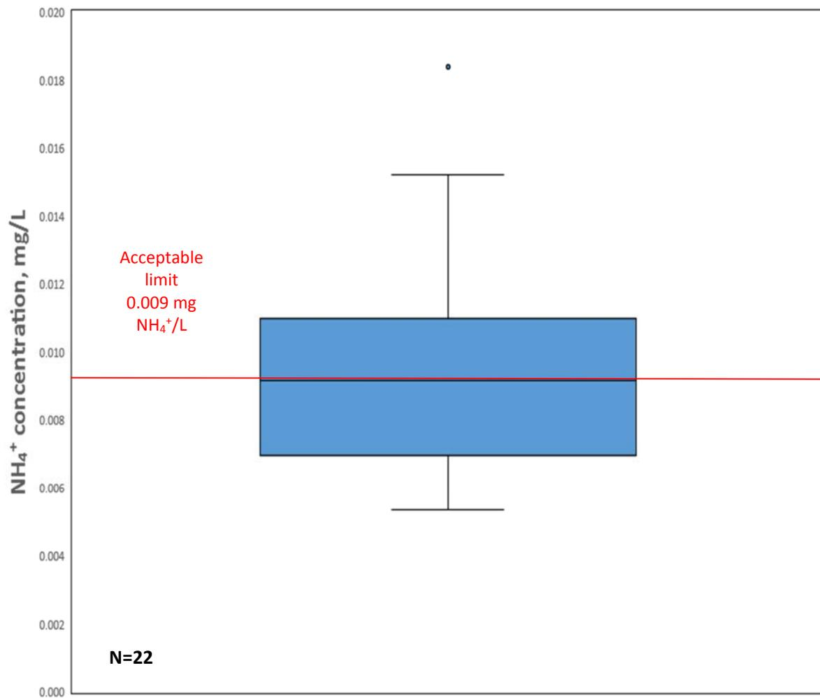
Figure 8. Box and whisker plot showing  $\text{NH}_4^+$  concentrations for new lids, tested with DI water in 2016
