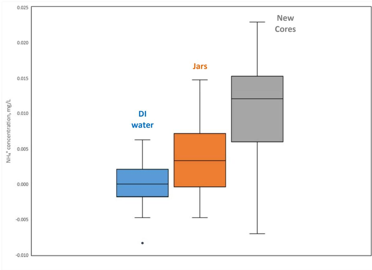
**Figure 12. Comparison of AMoN supplies blanks ( $\text{NH}_4^+$  concentrations, measured in DI water blanks, in washed and reused glass jars blanks and in new Radiello™ cores blanks) in 2016**
