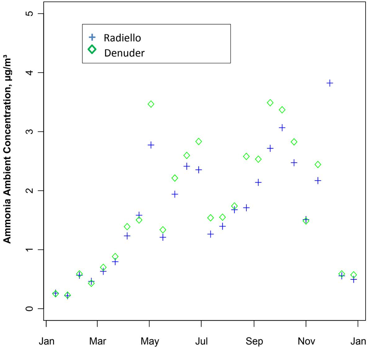
Figure 14. Ambient air concentrations of ammonia, measured at IL11 during 2016 using co-located Radiello™ passive samplers and URG™ denuders
