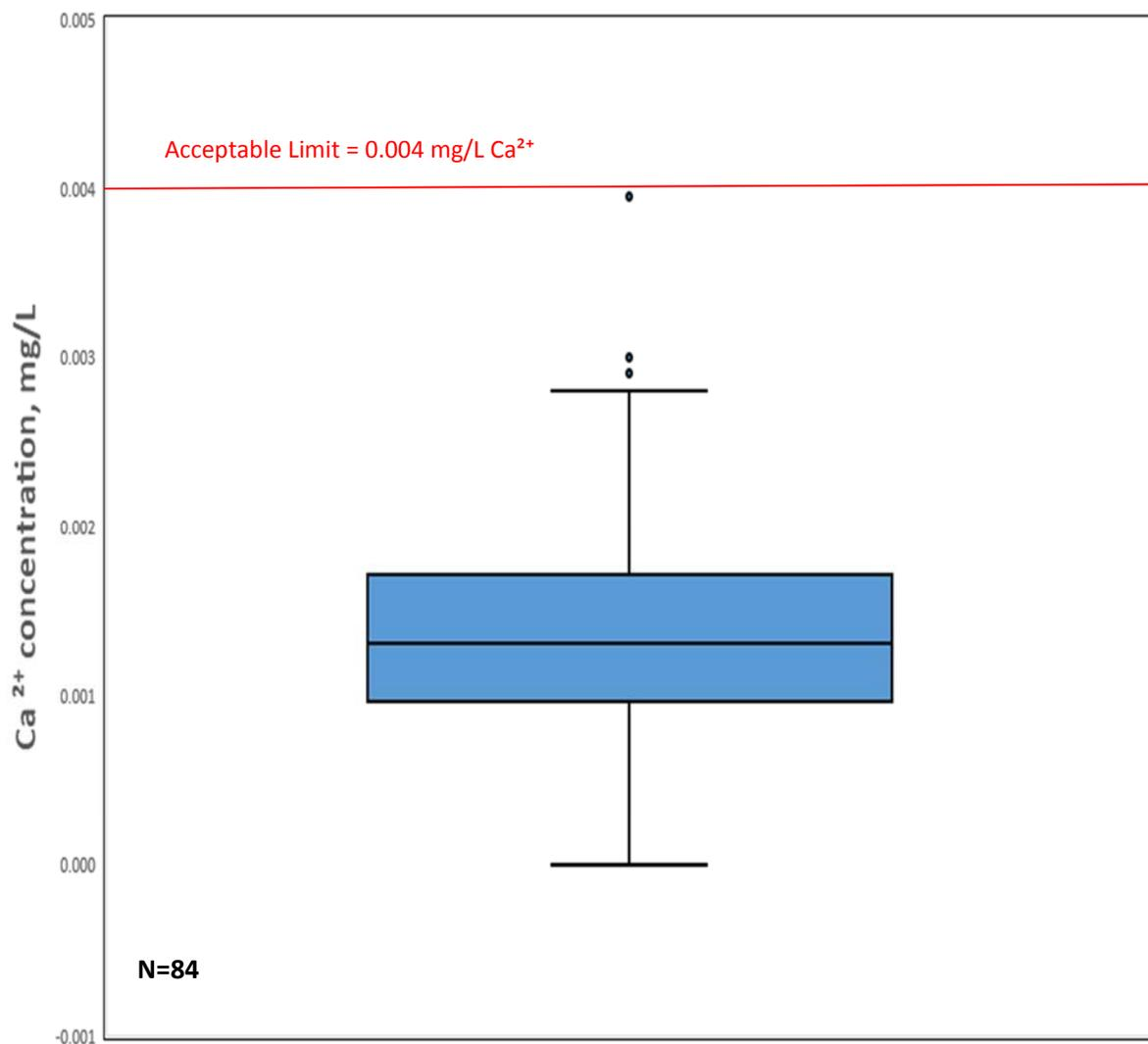
Figure 3. Box and whisker plot showing Ca<sup>2+</sup> concentrations for new buckets, tested with DI water in 2016
