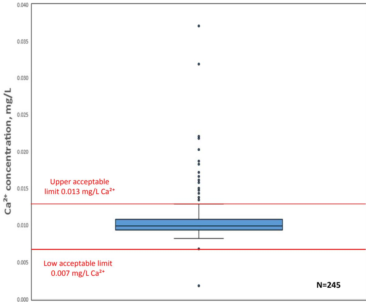
Figure 9. Box and whisker plot showing Ca<sup>2+</sup> concentrations for washed and reused bucket lids, tested with MDL solution in 2016
