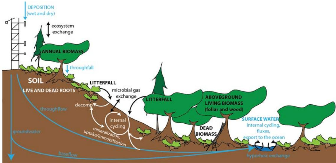
**Figure 6.** NEON biogeochemistry measurements within a site. Shown are variables that are part of the terrestrial biogeochemistry design (Terrestrial Observation System, TOS), as well as those associated with the tower (TIS), above- and belowground plant biomass (TOS), microbial community (TOS), and ground and surface waters (AOS/AIS). Subsurface hydrological flow paths that are important to constrain in biogeochemical budgets are shown, but will not be measured by NEON.
